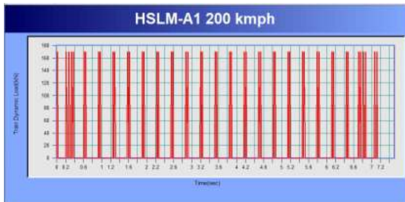
Fig. 7. Dynamic loading function from the load model HSLM-A1 200 km/h
