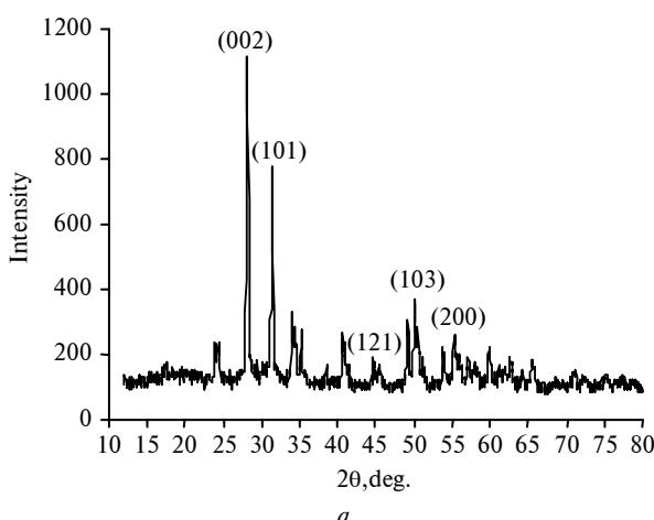
Fig. 1. Diffraction patterns of  $\text{ZrO}_2$  samples: *a* – sample 1, *b* – sample 2
