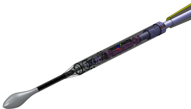
Fig. 4. Sketch of the model UA-2 and the support sting in MUB ISM
