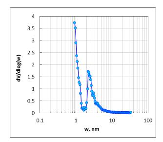
Fig.1. Pore size distribution for oxidized coal obtained from bagasse.
