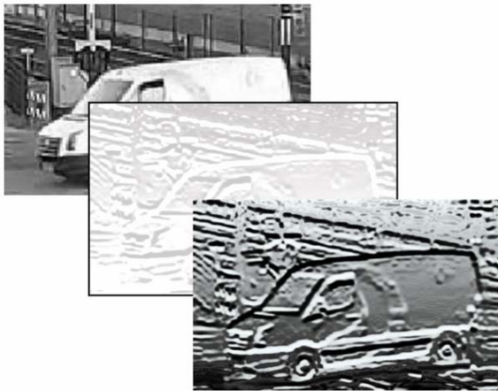
Fig. 3. Example of image processing by convolution cores
