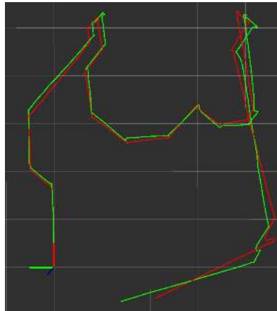
Fig. 2. - Robot's path respect to wheel odometry information (green) and estimated by EKF (red) [2].
