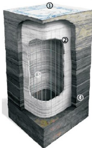
Figure 2. Three-dimensional renderings of the frozen wall 1 – Earth's surface; 2 – Frozen wall; 3 – Frozen Well; 4 – Oil shale
