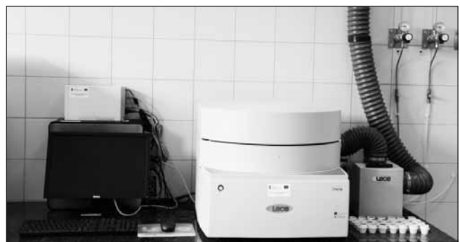
Fig. 3. LECO True-Spec (CHN module), own material
