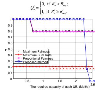
Fig. 3. Dependence of the probability of the required bandwidth capacity allocation to the UE for different methods of frequency-time resource allocation
