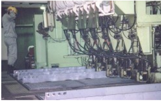
Fig. 1. Cutting of the flange plates from wide plates by flame.
