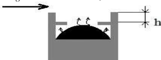
Fig. 9. Sketch of wagon with additional vertical boards “internal wings”
