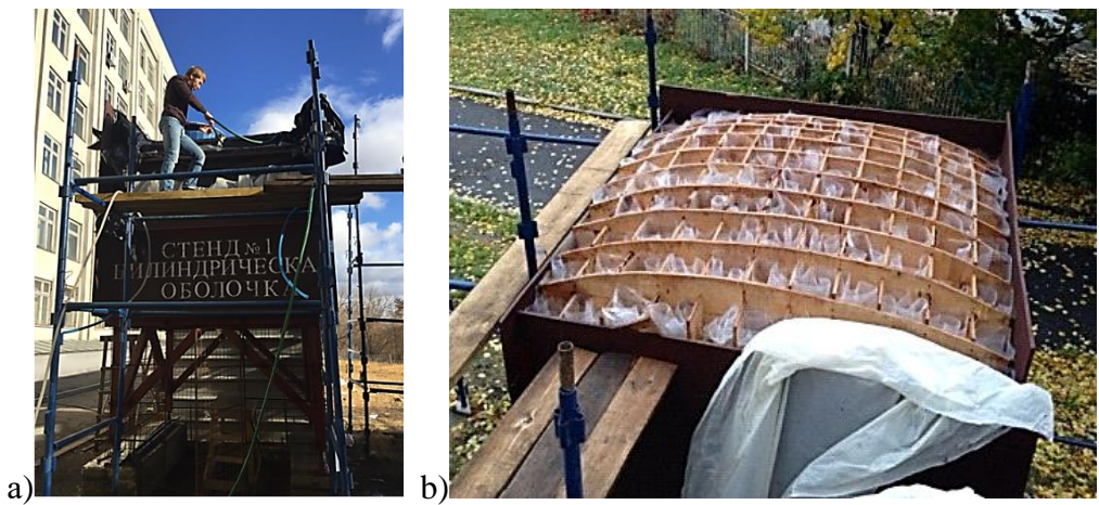
Fig. 2. Bench tests of shells: a) - water supply to the tank; b) - tank design
