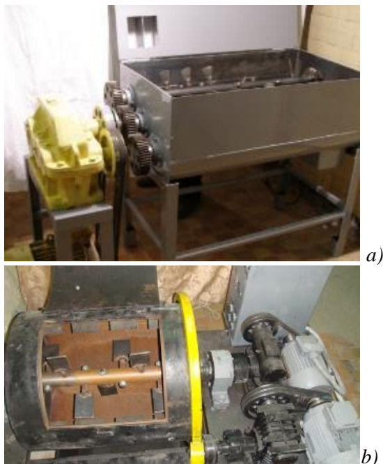
Fig. 1. Concrete mixers operating in cascade mode a) three-shaft; b) with gravity and forced action
