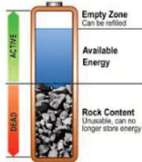
the process of a battery's "health" deterioration.
