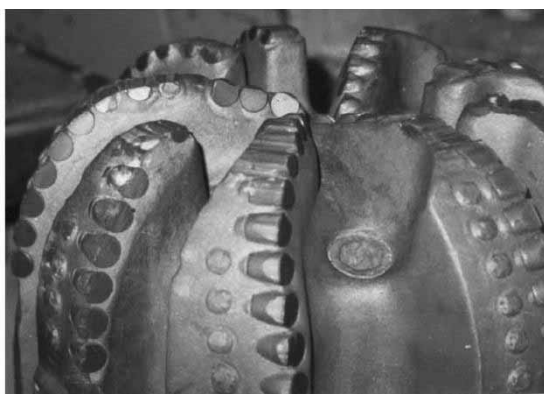
Fig. 5. Worn PDC cutters (drill bit-Read Hycalog 11 5/8 DS 66)
