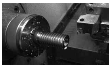
Fig. 2. The Worm Processing in the CN Lathes
