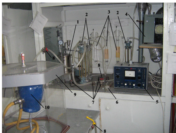
Fig. 4. Overall view of a stand: 1 – aerosol generator; 2 – rotameters; 3 – liquid micromanometers; 4 – an aspirator; 5 – an integral photometer; 6 – a three-way valve; 7, 8 – adjustable valves; 9 – a test chamber; 10 – special mounting to fix half-mask or dummy head (filters require mounting only)
