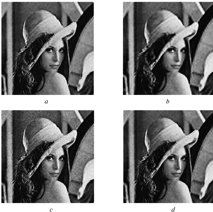
Fig. 7. Denoising Results of All Threshold Functions: a – Hard Threshold Denoising Results; b – Soft Threshold Denoising Results; c – Denoising Results of Fusion Threshold A; d – Denoising Results of Fusion Threshold B
