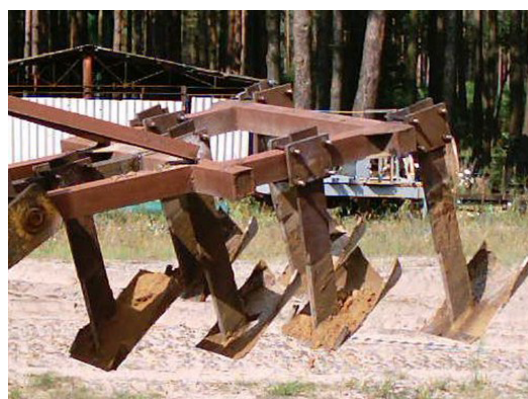
Fig. 4. Tiered operating units for deep soil differentiated tillage with improved stands:
