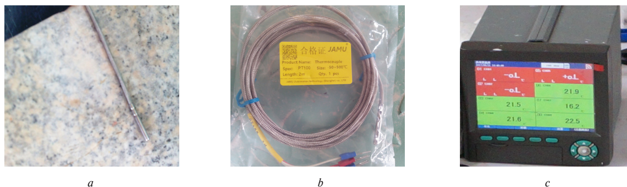
Fig. 1. Components of the measurement system used in the course of the experiments: sensor in the protection sleeve ( a ), illustration of the sensor ( b ), digital controller of temperatures ( c )
