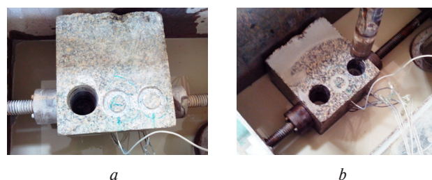
Fig. 3. Mining rock slab with mounted thermal sensors on the bench experiments table: a – before drilling; b – after drilling
