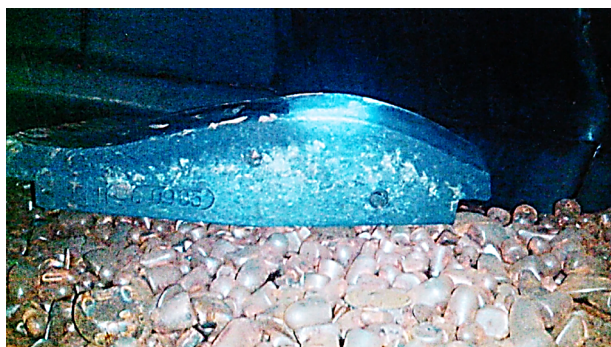
Fig. 7. Rubber lining of the “H-Wave Plate” type in the mill MIIIP 4.0 × 5.0 (the Poltava GOK Company, the first stage of grinding, iron ore, balls \varnothing 100 mm, t = 8891 h)
