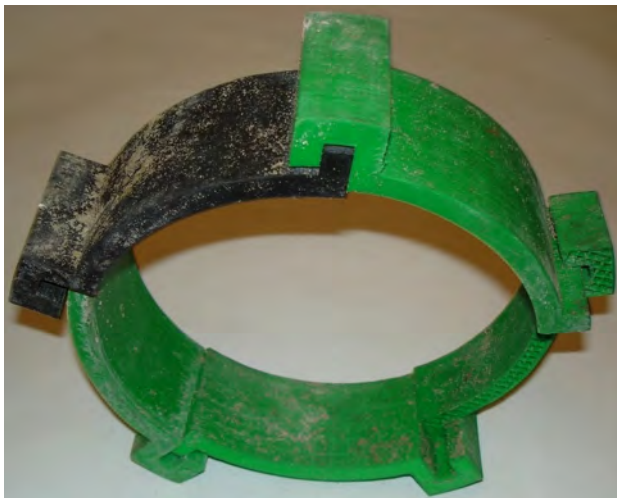
Fig. 1. A protective lining model sample with longitudinal joints of the clutch after testing in corrosive environment
