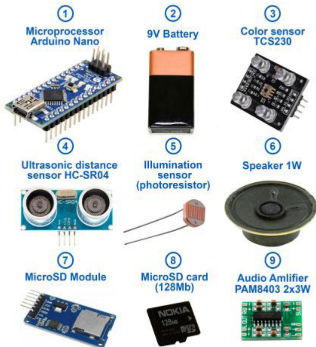
Fig. 2. Main device components
