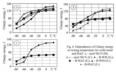
Toughness change subject to testing temperature in HAZ and weld metal carried out in MAG process with filled wire FW-10 (0.35% Ti) on the base metal Nb/Ti (C) and one level of heat input (E = 8.8 kJ/cm) is shown in Fig. 6*c*, and there is a large difference between toughness values in the HAZ and the weld metal.
