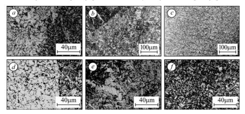
Fig. 4. HAZ microstructure of welded steel Nb/Ti-B:  $a-c - E_1 = 7.5$  kJ/cm;  $d-f - E_2 = 21$  kJ/cm.
