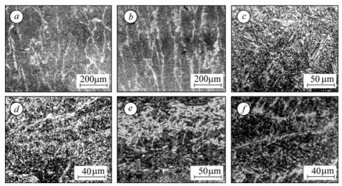
Fig. 1. WM microstructure in last pass of welded steels Nb/Ti (A, B) obtained with E-process using fillers N1, NM1, N2 and NM2: a – steel-A, FM-N1, E = 8.6 kJ/cm; b – steel-A, FM-NM1, E = 9.1 kJ/cm; c – steel-B, FM-N2, E = 11.5 kJ/cm; d – steel-B, FM-NM2, E = 7.5 kJ/cm; e – steel-B, FM-N2, E = 18.5 kJ/cm; f – steel-B, FM-NM2, E = 21 kJ/cm.
