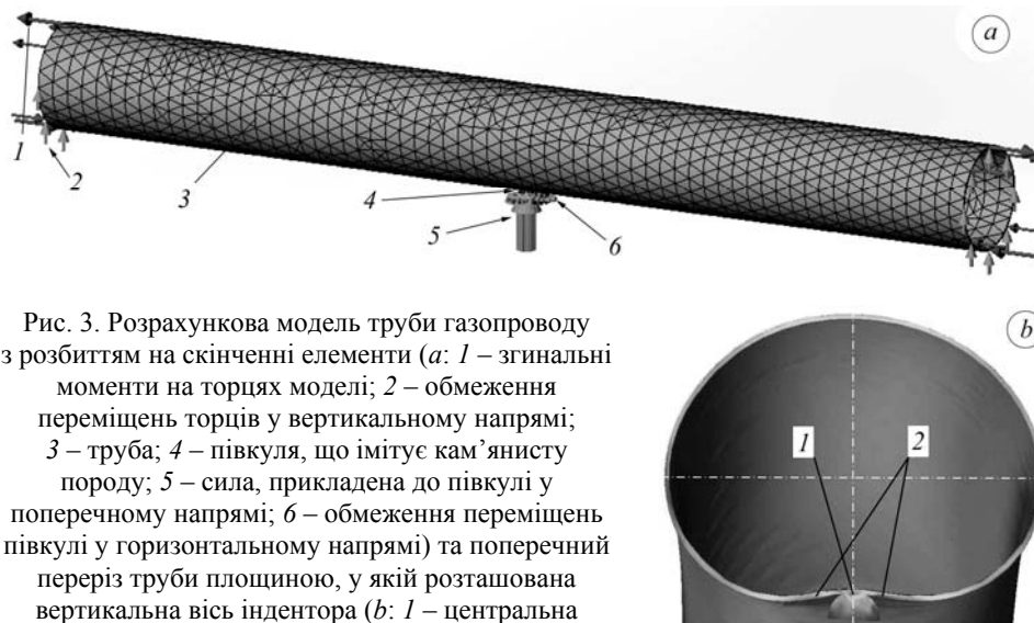
Fig. 3. Calculation model of a pipeline pipe divided into finite elements (a: 1 – bending moments at the ends of the model; 2 – limited movement of the ends in the vertical direction; 3 – pipe; 4 – hemisphere, simulating stony rock; 5 – force applied to the hemisphere in the transverse direction; 6 – limiting movement of a hemisphere in horizontal direction) and the cross section of the pipe by a plane with a vertical axis of indenter (b: 1 – central point of the contact zone; 2 – contour point of a dent).
