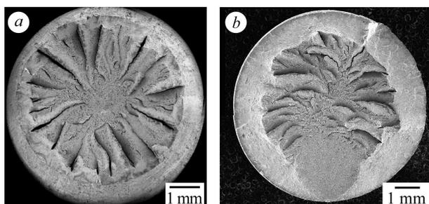
Fig. 3. Microfracture maps of steel E4 after tensile test in air (a) and under hydrogenation in the solution containing 1 g/l  $\text{Ca}(\text{OH})_2 + 0.1 \text{ g/l NaCl}$ , pH 12.5 (b).
