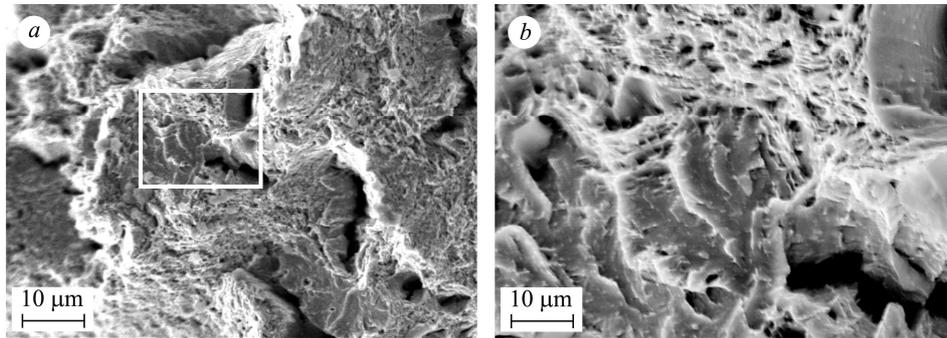
Fig. 5. Fracture surface of the prestressing steel wire central zone after the tensile test under hydrogenation in the solution with pH 12.5 (*a*) and its details (*b*).
