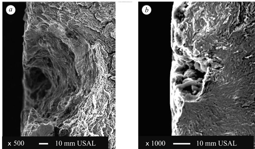
Fig. 3. Types of surface defects on the prestressing pearlitic steel.
