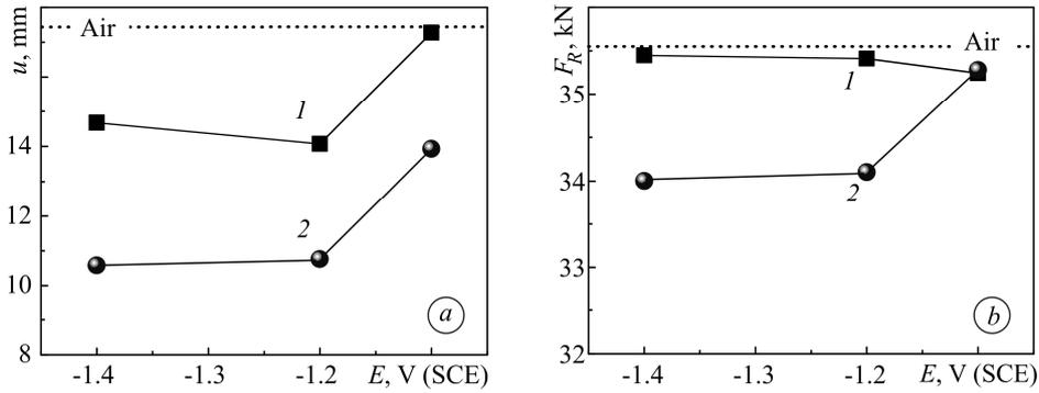
Fig. 2. Change in elongation to fracture  $u$  (a) and maximum load to fracture  $F_R$  (b) of the prestressing steel in SSRT under cathodic polarization with different strain rates:  $1 - 7.5 \cdot 10^{-6} \text{ s}^{-1}$ ;  $2 - 7.5 \cdot 10^{-7} \text{ s}^{-1}$ .
