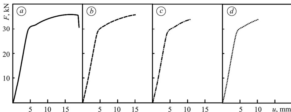
Fig. 1. Load-displacement curves of the prestressing steel in the medium containing 1 g/l  $\text{Ca}(\text{OH})_2$  + 0.1 g/l NaCl (pH 12.5) in air (a) and under cathodic polarization:  $-1.1 \text{ V}$  (b),  $-1.2 \text{ V}$  (c),  $-1.4 \text{ V}$  (d); strain rate  $7.5 \cdot 10^{-7} \text{ s}^{-1}$ .
