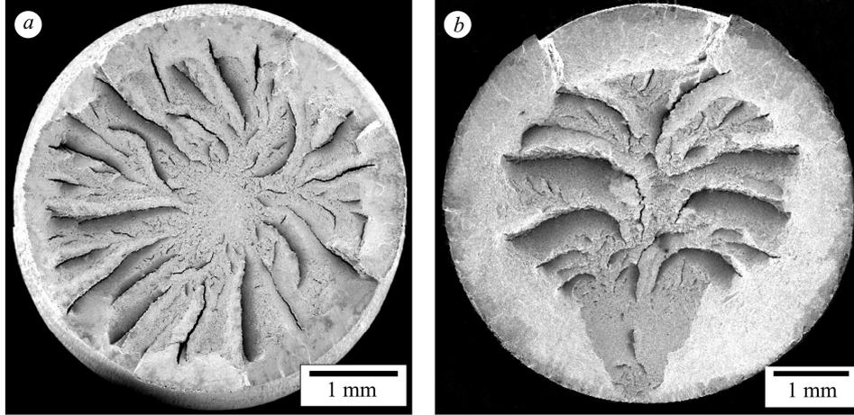
Fig. 4. Fracture maps of the prestressing pearlitic steel after the test in air [10] (*a*) and in alkali medium (pH 12.5) under cathodic polarization  $-1.2$  V (SCE) with a strain rate  $7.5 \cdot 10^{-7} \text{ s}^{-1}$  (*b*).
