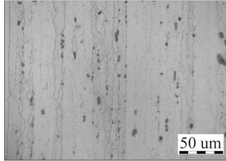
Fig. 2. Microstructure of 2017A-T4 alloy.
