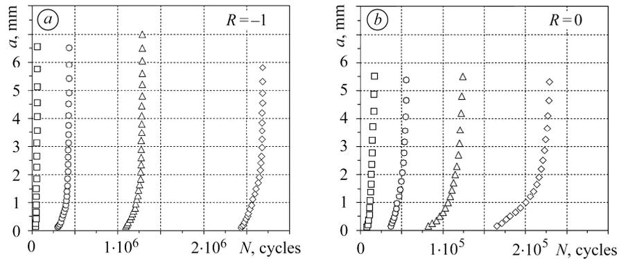
Fig. 5. Fatigue crack length versus number of cycles for different radii of the notch root for  $R = -1$  (a) and  $R = 0$  (b):  $\square$  –  $\rho = 0.2$  mm;  $\circ$  –  $\rho = 5$  mm;  $\triangle$  –  $\rho = 10$  mm;  $\diamond$  –  $\rho = 22.5$  mm.
