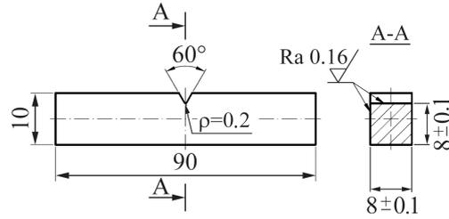
Fig. 1. Test specimen dimensions in mm.
