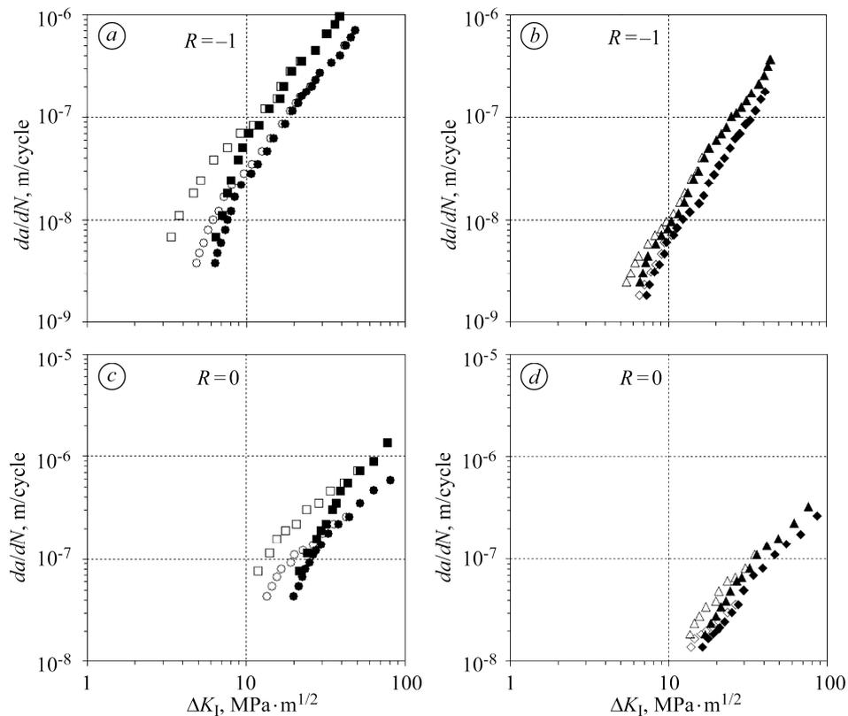
Fig. 6. Fatigue crack growth rate  $da/dN$  versus  $\Delta K_I$  with and without the correction factor  $Y_{2FR}$  for  $\rho = 0.2$ ; 5 mm (a, c) and  $\rho = 10$ ; 22.5 mm (b, d).
