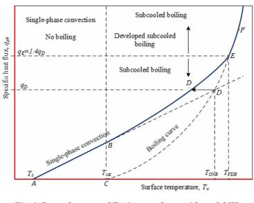
Fig. 1. Dependence  $q_{pb}=f(T_w)$  in accordance with model [7]
