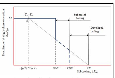
Fig. 2. Dependence of heat fraction at single-phase convection on subcoolings [7]
