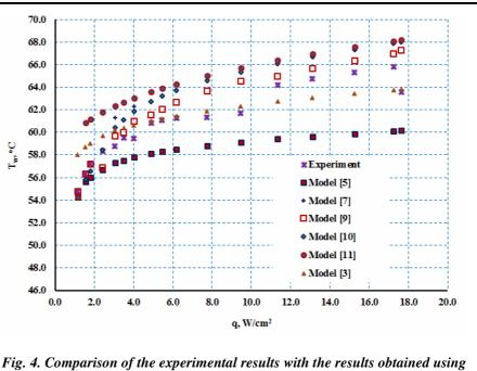
Fig. 4. Comparison of the experimental results with the results obtained using different models of heat transfer during subcooled boiling
