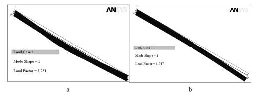
Fig. 3. Buckled shape and load factor for (a) simply supported and (b) cantilever beams.
