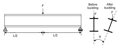
Fig. 1. Lateral torsional buckling at angle  $\theta$ .
