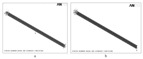
Fig. 2. Finite element model and boundary conditions for (a) simply supported and (b) cantilever beams.
