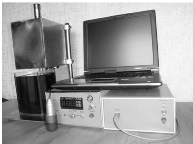
Fig. 3. Thermo – sonar system for measuring cooling intensity of liquid quenchant.
