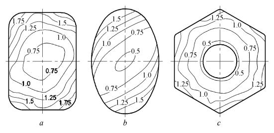
**Fig. 6.** Distributions of Von Mises equivalent strain in cross-section of billets having rectangular (a), oval (b) and hexagonal with hollow centre (c) profiles
