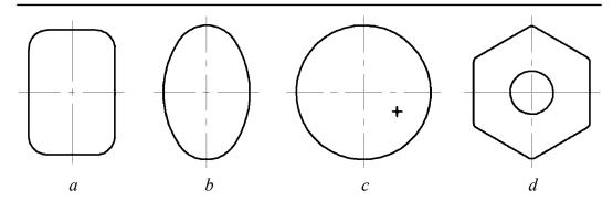
**Fig. 2.** A few examples of cross-sections of dies for twist extrusion: a – rectangular; b – elliptical; c – circular, '+' denotes the position of extrusion axis; d – hexagonal with a hollow centre
