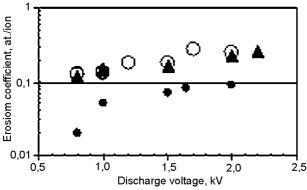
Fig. 2. Erosion coefficient dependence on nitrogen ion energy for Pd-W systems:  $\blacktriangle$  – dense W film, o – W film of the 45% porosity,  $\bullet$  – experimental data for hydrogen saturated W films [2].
