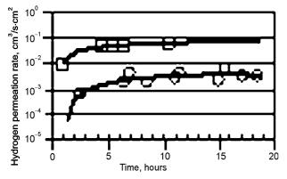
Fig. 6. Hydrogen permeation rate measured at 973 K temperature and at hydrogen pressure of  $10^5$  Pa versus time of baking at 973K temperature:  $\Box - 4 \mu m$  VPD W-film on Pd,  $o - 300 \mu m$  CVD W-film on Pd.
