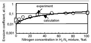
Fig. 3. Tungsten erosion coefficient versus nitrogen concentration in hydrogen: experimental data for 1.2 keV ion irradiation (o), curve is the calculated data.
