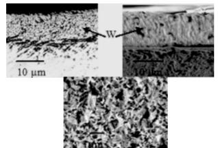
Fig. 1. The metallographic microscopic sections (left, center – before and after annealing) and surface morphology (right) of 15  $\mu$ m W film deposited at Ar pressure of 10.4 Pa.
