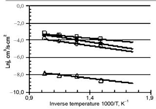
Fig. 5. Temperature dependencies of specific hydrogen flow through two-layer Pd-W systems at  $10^5$  Pa H<sub>2</sub> pressure: bare palladium ( $\Box$ ); high porous 14 µm and 9 µm W film on Pd ( $\triangle$ ,  $\blacktriangle$ ); 4 µm dense W film on Pd ( $\Diamond$ ).
