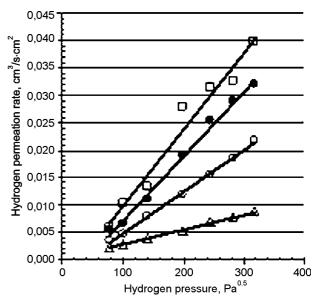
Fig. 4. Hydrogen permeation rate at 973 K temperature versus pressure: bare palladium ( $\Box$ ); high porous 14  $\mu$ m, 9  $\mu$ m W film on Pd ( $\triangle$ ,  $\blacktriangle$ ); 4  $\mu$ m dense W film on Pd ( $\Diamond$ ).
