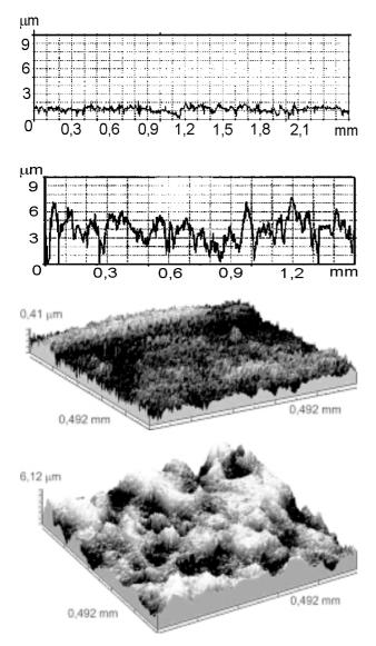
Fig. 2. Three-dimensional AFM images of the initial sample surface (1) and the deformed sample surface (2).
