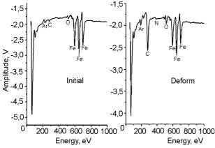
Fig. 5. Auger-spectra of the initial (on the left) and the deformed (on the right) samples surfaces.
