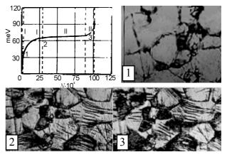
Fig. 1. The kinetic fatigue curve and the photos of microstructures corresponding to observation points 1, 2, 3 on the curve.
