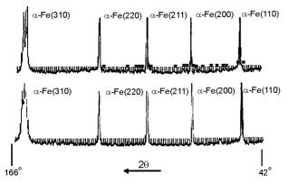
Fig. 7. X-ray diffraction pattern deformed samples (1) and the initial samples (the lower one).
