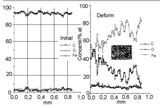
Fig. 4. AES-depth profiles of the initial sample surface (on the left) and the deformed sample surface (on the right).
