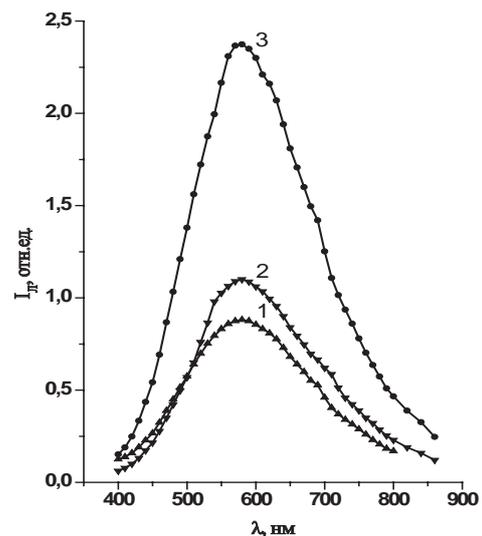
Fig. 2. Luminescence spectrums of NC CdS (sample № 1) at various excitation power, mWt: 26,6 (1) 19,5 (2); 45,0 (3).
