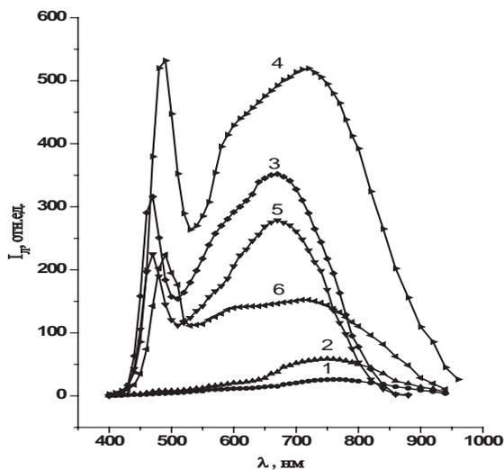
Fig. 3. Luminescence spectrums of NC CdS (sample № 2) at various excitation power, mWt: 19,5 (1); 26,0 (2); 32,0 (3); 42,0 (4); 45,0 (5); 26,6 (6).
