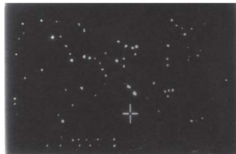
FIG. 1. Image of artificial stars given by the sensor (250x250 pixels)
