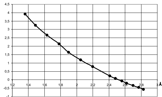
Fig. 3. The changes of the total energy of two diamond-like carbon films with a mixture of 50% the diamond-like and 50% the graphite-like bonds versus the change of the separation distance between films D. Energy is supplied in atomic units per atom, distance - in Å.
