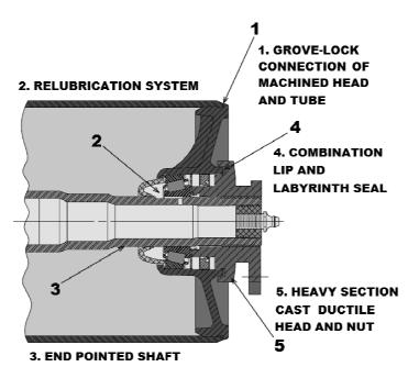
Fig. 6. SDX-Plus sealing system from Joy Mining Machinery
