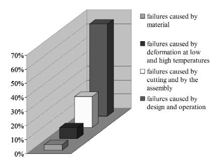
Fig. 3. Causes and weight percentage of failures due to fatigue
