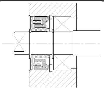
Fig. 5. Sealing system with double labyrinth
