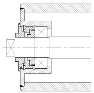
Fig. 4. Sealing system with simple labyrinth
