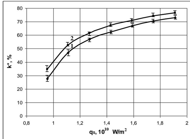
Fig. 3. Graph charts of the experimental dependence  $k^* = k^*(v)$  during marking with fiber laser SP – 40P done on sample of carbon tool steel Y11:
