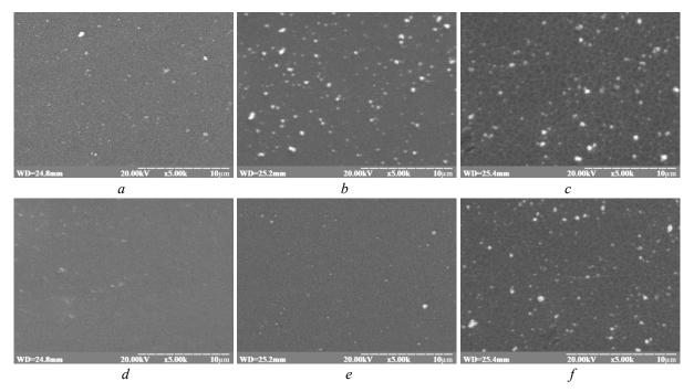
Fig. 4. The surface morphology of ZnS films obtained using trisodium citrate with different deposition duration (a -80 minutes, b -100 minutes, c -120 minutes) and with different deposition temperatures (d -50 °C, e -70 °C, f -90 °C)
