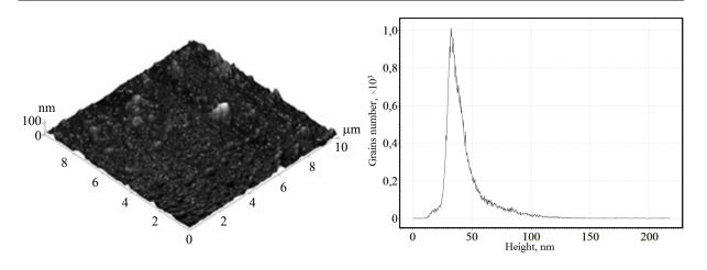
Fig. 5. The three-dimensional AFM image of the surface and the distribution histogram of the crystal grains height above the surface of the ZnS films using optimum conditions
