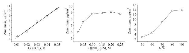
Fig. 2. The change dependence of zinc weight per unit area in ZnS films on the initial concentration of zinc-containing salt, the concentration of thiourea and deposition temperature
