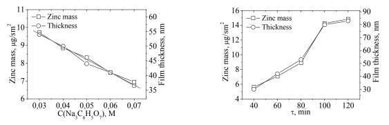
Fig. 3 The change dependence of zinc weight per unit area and the thickness in ZnS films on the concentration of sodium citrate and duration of the precipitation
