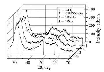
Fig. 1. The experimental profiles of diffraction patterns of ZnS films obtained from different zinc salts and their comparison with the lines of theoretical diffraction pattern of ZnS
