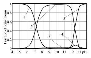
Fig. 2. Ratio of dissociated forms of orthoboric acid in the coolant: 1 – molecular form of H<sub>3</sub>BO<sub>3</sub>; 2 – anion of the first degree of the association H<sub>3</sub>BO<sub>3</sub>OH<sup>-</sup>;
