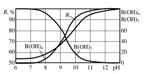
Fig. 3. Selectivity of Filmtec and Hydranautics membranes in relation to boron, depending on the pH of the solution
