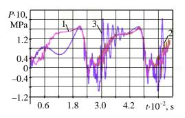
Fig. 6. Change in pressure in the working cavities of the HPD of vibro-impact device: 1 – in the cavity of the executive hydraulic cylinder;
