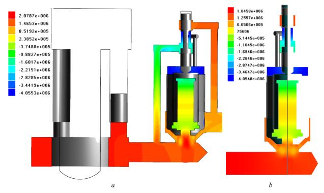
Fig. 4. Distribution of pressure in the working cavity of the HPD of the vibro impact device: in the y0x plane (a); in the z0y plane (b)
