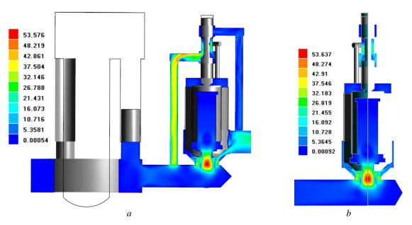
*Fig. 5. Distribution of speed in the working cavity of the GIP of the vibro impact device: in the y0x plane (a); in the z0y plane (b)*
