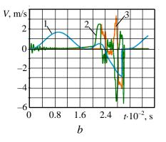
*Fig. 7. Diagrams of changing the working parameters of the HPD: changes in displacement (a); change of speed (b); 1 – impact mass; 2 – the valve of the first cascade; 3 – the valve of the second cascade*
