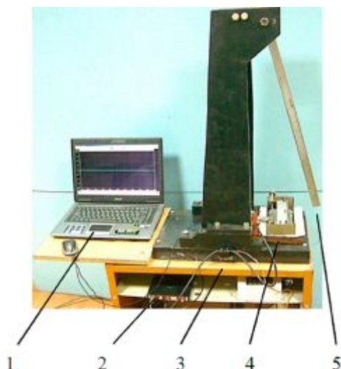
Fig. 7. Equipment for determining the DBTT based on the recording of AE signals (without a thermostat): 1– computer; 2 – Handyscope HS measuring instrument; 3 – signal amplifier AE; 4 – module for moving the sample; 5 – striker
