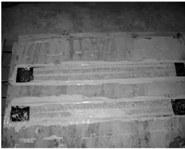
(a) Specimen S-2 (strengthened with AS4 3501)
