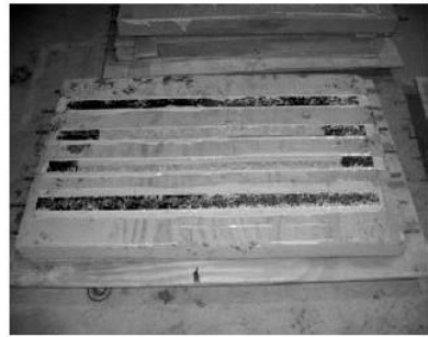
(b) Specimen S-4 (strengthened with AS4 3501)
