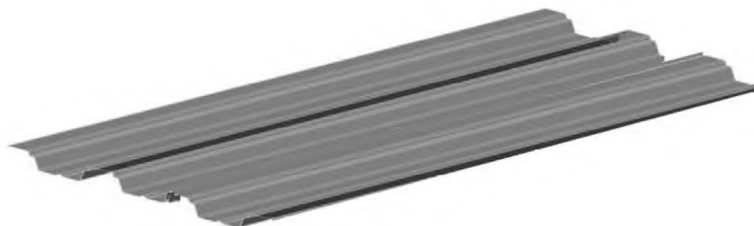
Fig.1. Three-dimensional geometrical modelling of profiled sheeting H75J
