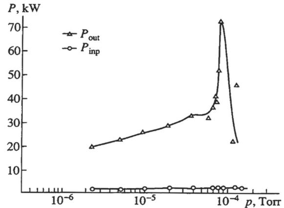
Fig. 3. Pulse power vs. working gas pressure
