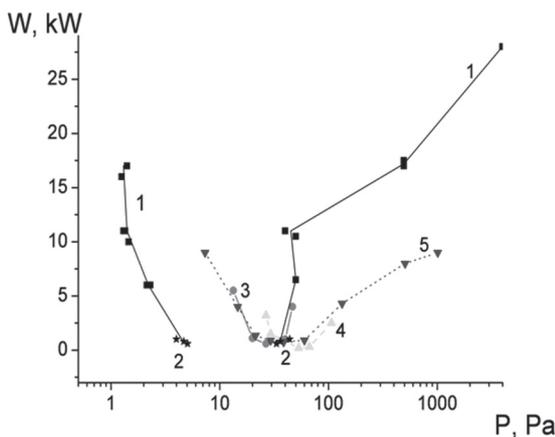
Fig. 11. Dependences for breakdown power of a microwave signals with a stochastically jumping phase versus a pressure for air in the optimal BPG mode (curves 1 – ■, 2 – \*), in the non-optimal BPG mode: for air (curve 3 – ●), argon (curve 4 – ▲), helium (curve 5 – ▼), respectively, at narrowband signal
