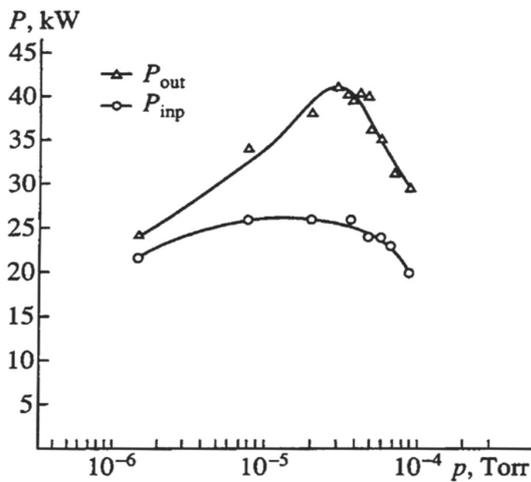
Fig. 2. Pulse power vs. working gas pressure
