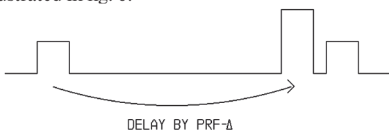
Fig. 6. Principle of a DRFM - Used to Create An Up-Range False Target
