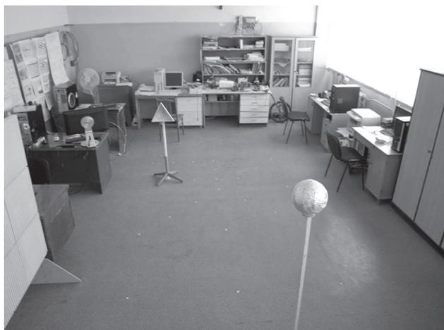
Fig. 3. Scenario for tomographic 3D SAR imaging
