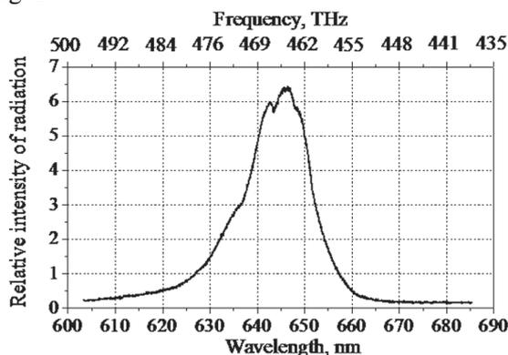
Fig. 2. Radiation Spectrum of the Toshiba TLRH190P LED
