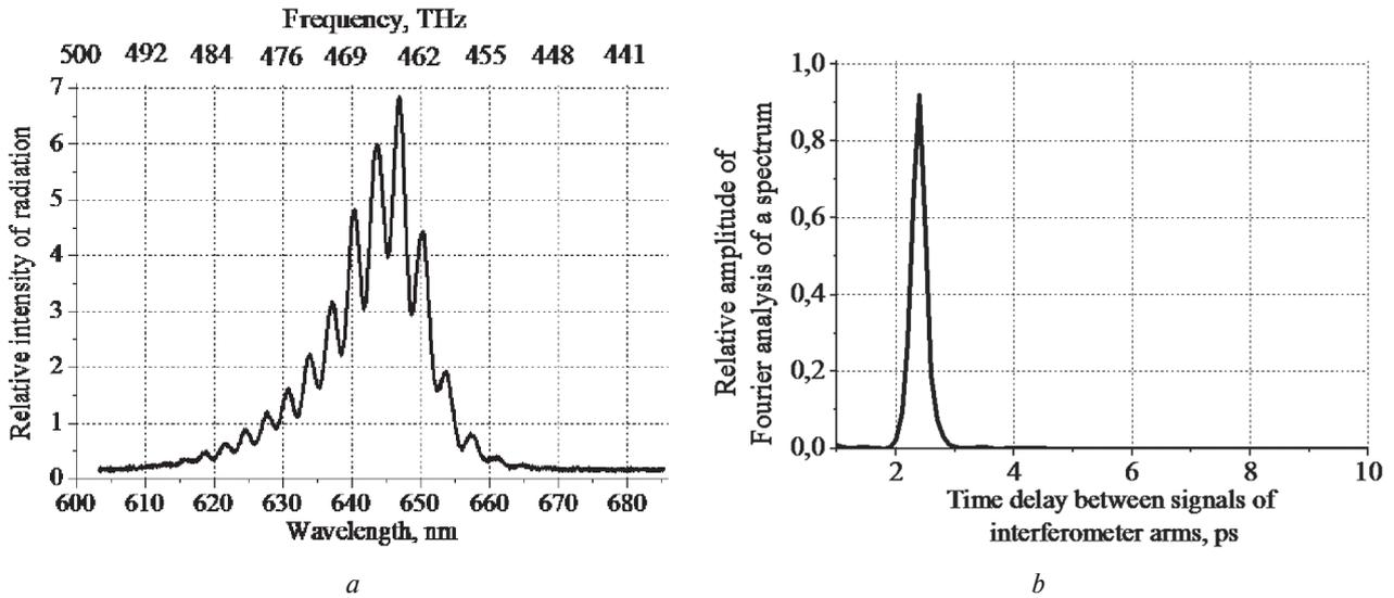
Fig. 4. *a* — Power spectrum of noise optical radiation of the Toshiba TLRH190P LED at the output of the Michelson interferometer: the arms difference exceeds the coherence length of the LED noise radiation; *b* — the result of the second Fourier transform being applied to the spectrogram of fig. 4a
