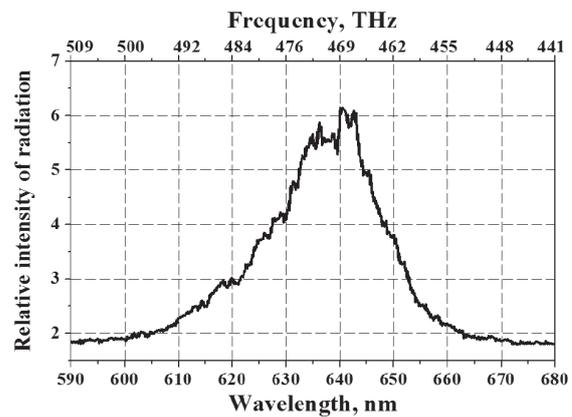
Fig. 3. Radiation Spectrum of the OptoSupply OSHR5111P LED
