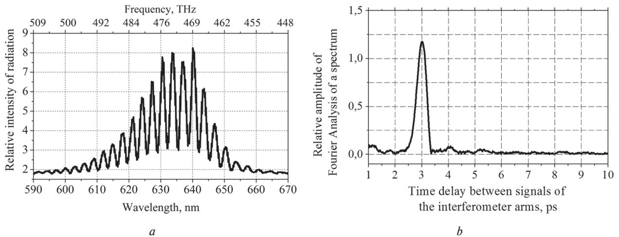
Fig. 5. *a* — Power spectrum of noise optical radiation of the OptoSupply OSHR5111P LED at the output of the Michelson interferometer: the arms difference exceeds the coherence length of the LED noise radiation; *b* — the result of the second Fourier transform being applied to the spectrogram of fig.5a.
