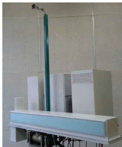
Fig. 5. Ground Based Noise Waveform SAR with horn transmit antenna
